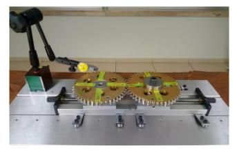
Fig. 14. Test rig & dial indicator.
