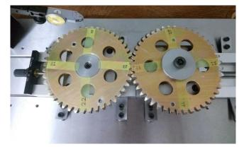
Fig. 15.Test spur gear pair & 4 main cases.
